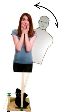
Target will swing out to the right then back into the concealed position.
