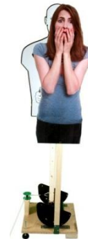
When target reaches concealed position, re-apply tension to hold it in place.
